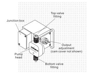
DOSING STAR $^{\text{TM}}$  dosing pump is designed to dose chlorine to the swimming pool in a safe and controllable way. It can helps avoiding direct contact with the chlorine tablets.
